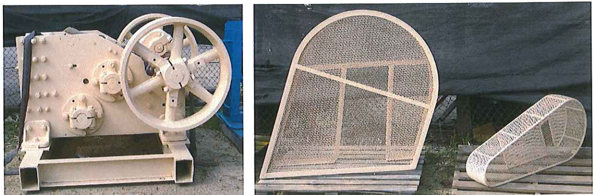
Figure 1.2 Cleaned and repainted jaw crusher. Mesh safety guards on right.
