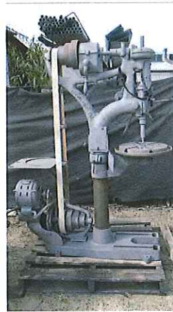
Figure 1.5 Drill press cleaned and ready for repainting.
