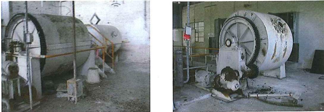
Figure 2.2 These ball mills contain heavy iron balls for crushing rock to powder to make glazes or to crush clay to a fine powder.
